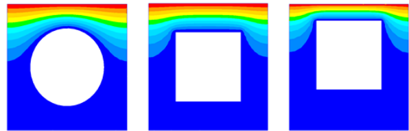
Figure 4. Temperature profile on the normal face for several geometries. Red is hot and blue is cold.
