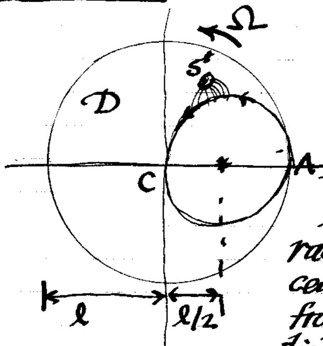
A spider moves in a circular path on the surface of a rotating disk. The path is fixed with respect to the disk hence rotates with it! The disk radius is ~~is~~  $l$  and the path radius is  $l/2$  with center at a distance  $l/2$  from the center of the disk. Assume that at  $t=0$
