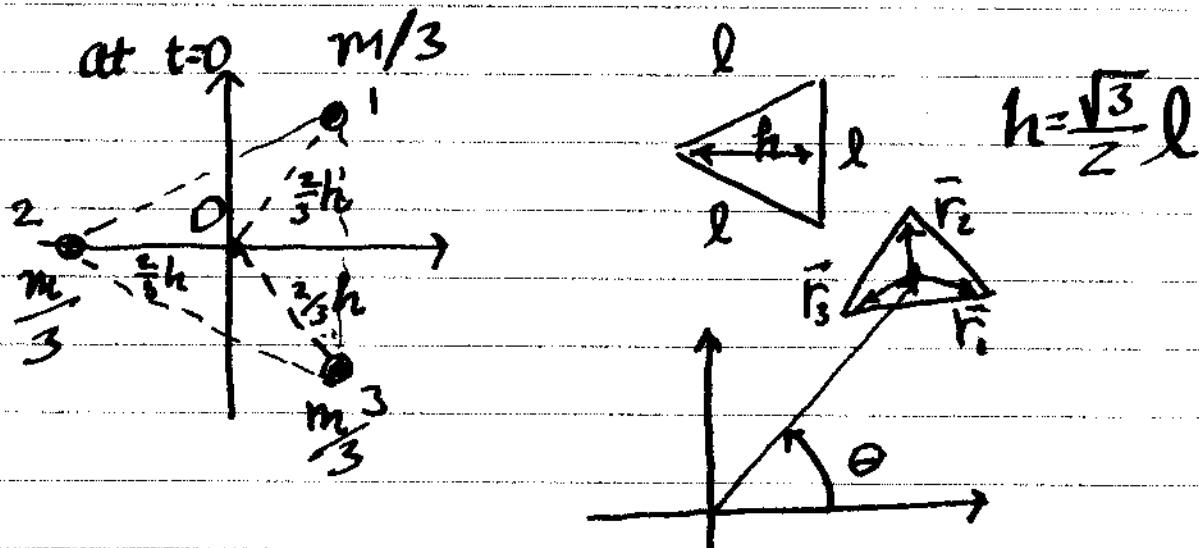
Three point masses are constrained to be at the vertices of an equilateral triangle of side  $l$ . In terms of the height  $h = (\sqrt{3}/2) l$  we chose a point 'O' equidistant from each of the three equal mass points. So the position of the three points are given at  $t=0$  by.
