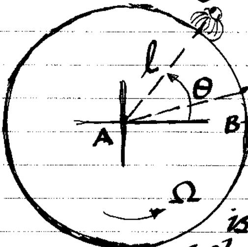
A spider is located at position  $s$ , given by  $le^{i\theta}$  in complex notation, relative to the point 'A' fixed in space. The spider moves along the rim with velocity  $v_s$  on the (relative to) the disk which is itself rotating with angular velocity  $\Omega$ . At  $t=0$  both the spider and the line  $AC$  (fixed on the disk) are at  $B$ , i.e.  $s, c$ , and  $B$  are coincident.
