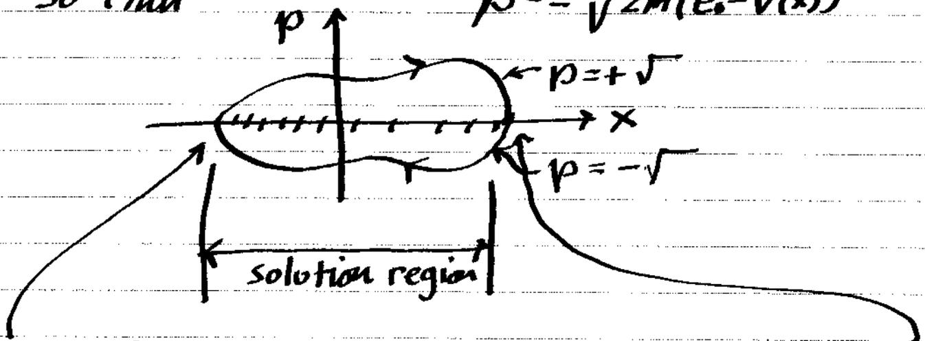
$V(\bar{x}) = E_0, p = 0$ , equation for turning point
