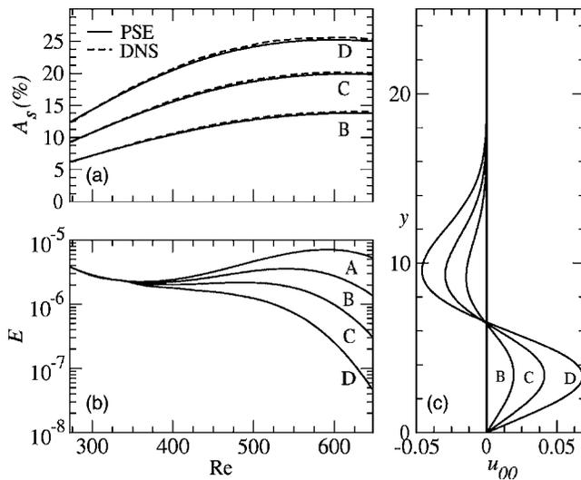
FIG. 1. (a) Comparison of DNS and PSE simulations of the nonlinear downstream development of three streaks with increasing amplitudes. (b) The evolution of the TS-wave in presence of streaks. (c) The mean-flow distortion at  $Re=640$  caused by streaks.
