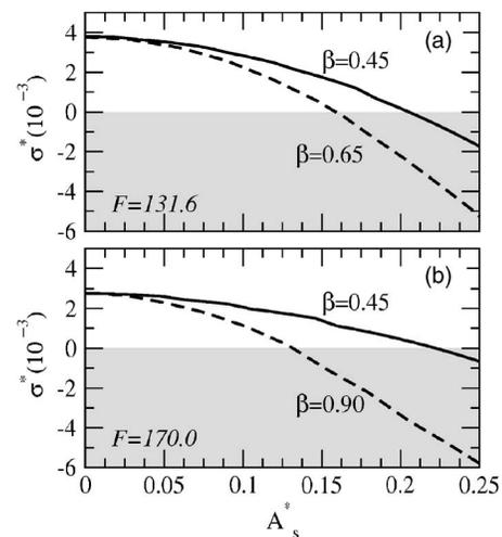
FIG. 4. The maximum growth rate  $\sigma^*$  of TS-waves,  $F=131.6$  in (a) and  $F=170$  in (b), in the presence of streaks.
