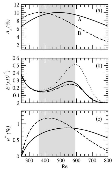
FIG. 2. (a) Evolution of amplitudes of two streaks with  $\beta=0.45$  (solid) and  $\beta=0.65$  (dashed). (b) TS-wave with  $F=131.6$  in absence (dotted) and presence (dashed, solid) of streaks. (c) The maximum value of the mean flow distortion caused by the streaks.
