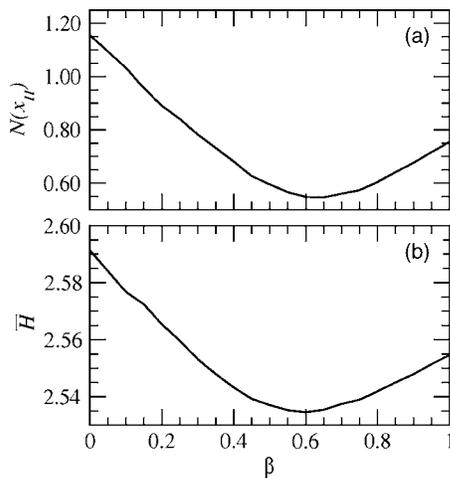
FIG. 3. (a) The  $N$ -factor at branch II of the TS-wave ( $F=131.6$ ) as a function of the spanwise wavenumber of streaks. The maximum amplitudes of the streaks have been fixed at  $A_s^*=10\%$ . (b) The averaged shape factor  $\bar{H}$  as a function of the same set of streaks as in (a).
