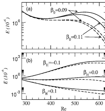
FIG. 5. (a) The downstream development of oblique waves ( $F=131.6$ ) in the absence (solid) and the presence (dashed) of streaks. (b) The downstream development of a TS-wave ( $F=131.6$ ) in the absence (solid) and the presence (dashed) of streaks in boundary layer with adverse, zero and favorable pressure gradient.
