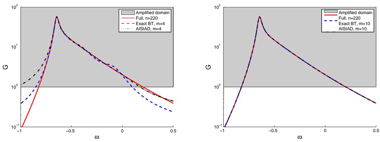
Figure 1: A comparison of the frequency response of the full model (red), the exact balanced truncation model (blue dashed) and the AISIAD-based model (black dashed dotted). The reduced system consists of a dimension of  $m = 4$  (left) and  $m = 10$  (right). The gray region marks the amplified frequencies.
