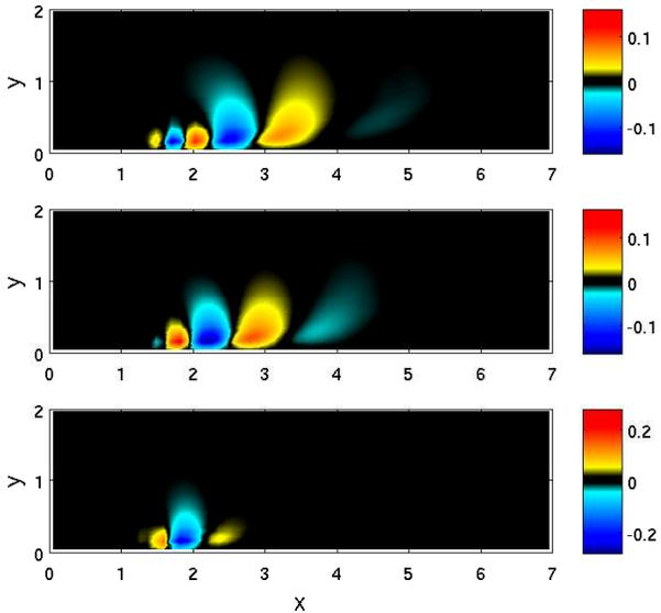
Figure 4: First three computed balanced modes  $S_c$  using the AISIAD method ( $m = 4$ ). The  $\tilde{v}$  velocity is displayed.
