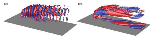
FIGURE 3. Positive (red) and negative (blue) contour levels of the streamwise velocity components of two Koopman modes. The wall is shown in grey. (a) Mode 2, with  $||v_2|| = 400$  and  $St_2 = 0.141$ . (b) Mode 6, with  $||v_6|| = 218$  and  $St_6 = 0.0175$ .
