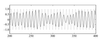
FIGURE 4. Comparison of time coefficients: the projection of the flow field onto the most energetic POD mode (black), and the coefficient of the most energetic Koopman mode (grey).
