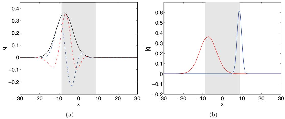
**Figure 1.** (a) The real part (dash-dotted line), imaginary part (dashed line), and the absolute value (solid line) of the optimal disturbance used as the input ( $B$  matrix in (2.6)) in the convectively unstable case. (b) The absolute value of the  $B$  matrix (red) and  $C$  matrix. In both (a) and (b), the grey region indicates the region defined by (2.4) where disturbances are amplified.
