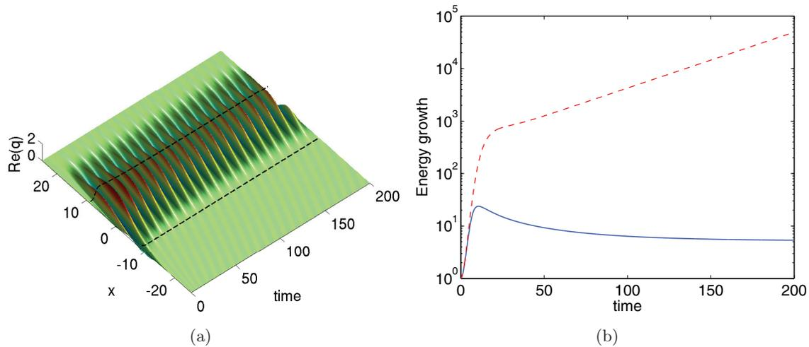
**Figure 5.** (a) The spatiotemporal nonlinear evolution of the optimal disturbance in the limit cycle case (real part). (b) The energy norm for the linear (red dashed line) and nonlinear (solid line) evolution of the CGL equation for the same case. In the linear case, the energy grows exponentially due to the unstable mode after the initial transient, while the limit cycle develops in the nonlinear case.
