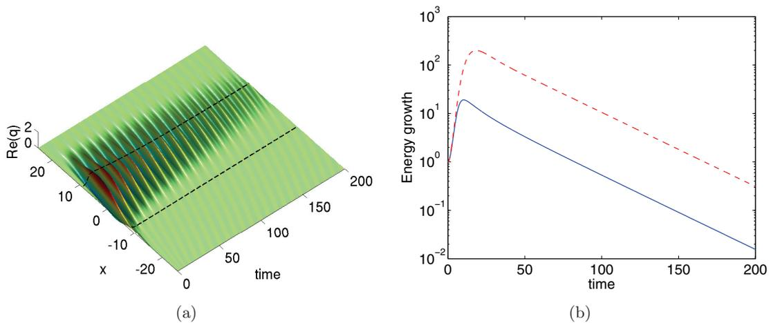
**Figure 2.** (a) The spatiotemporal nonlinear evolution of the optimal disturbance in the subcritical case (real part). (b) The energy norm for the linear (red dashed line) and nonlinear evolution of the CGL equation (solid line) for the same case. The transient nonnormal growth of the nonlinear solution is considerably smaller compared to the linear case due to the nonlinear damping.
