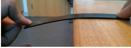
FIGURE 1.3. An example of a deformed ruler. A force is applied at both ends of the ruler and at center of the ruler (reactive force from table), which causes a bending of the ruler.
